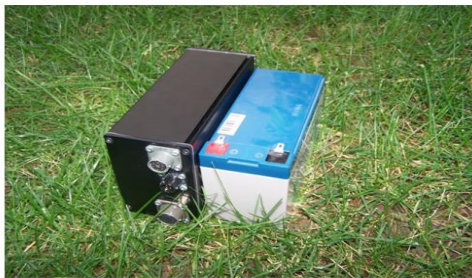
Figure 5: Photo of a new generation 32bit PST seismograph developed by Landtech-Geophysics and Geobit. It is powered by a motorcycle battery for more than a month.
