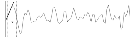
Figure 8: Measurement of rise time and pulse width broadening.
