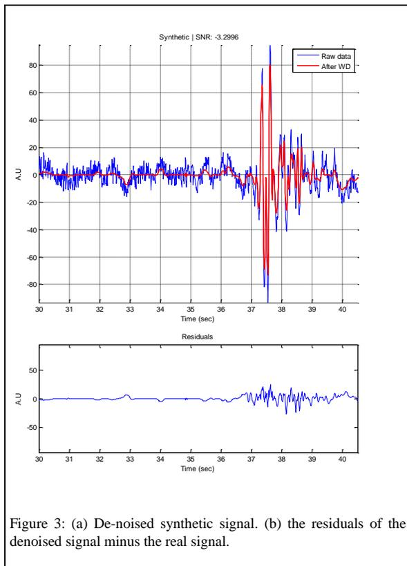
Figure 3: (a) De-noised synthetic signal. (b) the residuals of the denoised signal minus the real signal.
