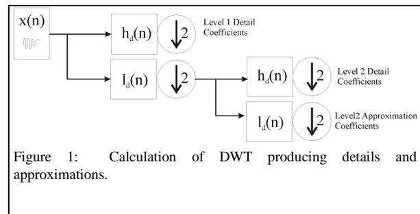
The wavelet coefficients represent a measure of similarity in the frequency content between a signal and a chosen wavelet function (Misiti, et al., 2009)
