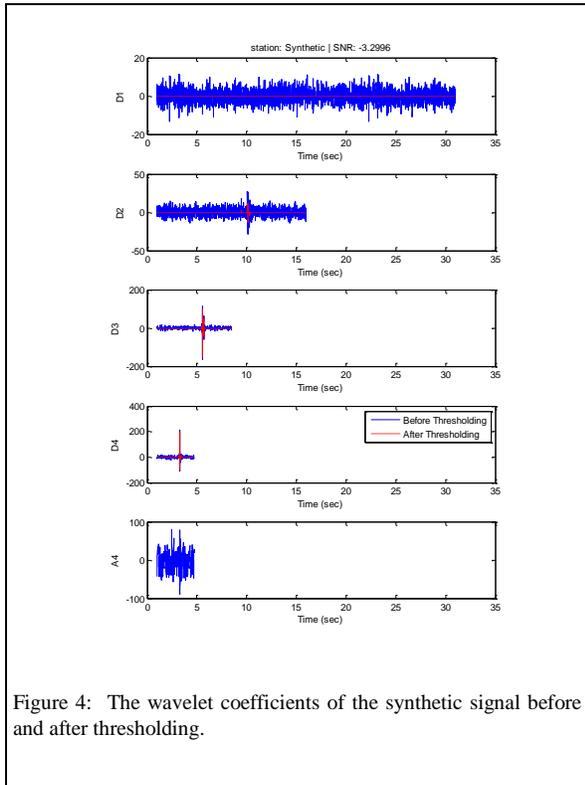
Figure 4: The wavelet coefficients of the synthetic signal before and after thresholding.
