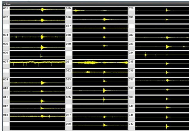
Fig.4. Example of an event recorded in most of the stations of the seismological network.
