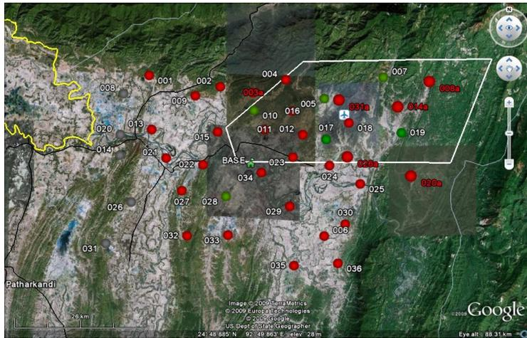
Trillium 40, three component sensors. The network spans an area of approximately 1900 km<sup>2</sup> covering the most of VC block area in order to ensure complete subsurface coverage (Fig.2). Recording began on 19<sup>th</sup> of November 2009 and completed on the 23<sup>rd</sup> of February 2010.
