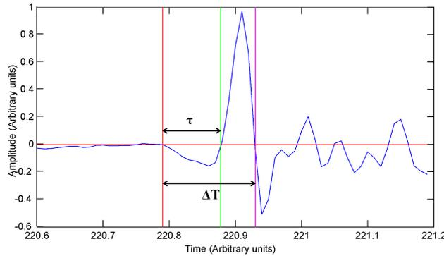
Figure 1: Rise time  $\Delta T$  and pulse width  $\tau$  of a seismic phase on a velocity seismogram
