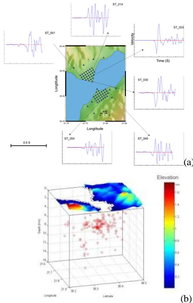
Figure 2: (a) Seismic station layout (triangles) and some velocigrams of the first breaks recorded from a local microearthquake (shown in 6 stations) The time segment shown is the same for all velocigrams (b) 3D distribution of microearthquake hypocenters recorded by the local network
