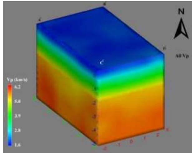
Figure 3: The 3D  $V_p$  (P wave) velocity model obtained from travel time tomography.
