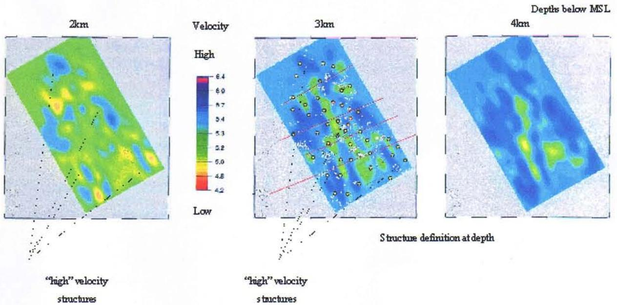
The results gave indications about carbonate and clastic velocities, which were converted into density information, incorporated into gravity and supported potential modeling.
