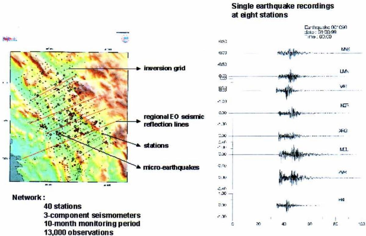
Manual P and S phase picking using PSL's "SEISMWIN" was performed, and the data were subsequently incorporated for hypocenter and earthquake parameter calculations.
