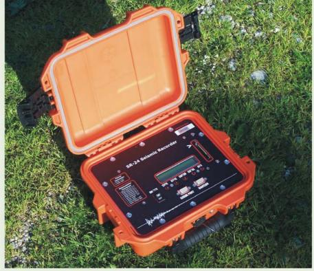
The SR-24 has 3 input channels, and capability for connection to a wide range of sensors. The digitizer is based on a powerful, wide dynamic range delta-sigma analog-to-digital converter, with very low noise characteristics and excellent power supply rejection. The sampling rate can be set to 40, 50, 60, 100, 125, 150, 200, 250, 300, 400 and 500 samples per second. Optional, sampling rates of 1, 2, 5, 10, 20, 25 and 600, 700, 750,1000 samples per second can be supported.
